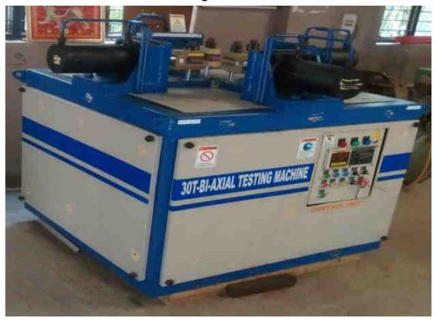
Flexural Fatigue Machine (Designed & Fabricated in house – lab). A testing equipment for research & testing purpose.
