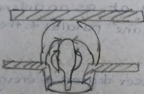
fig: probe coupling in a rectangular waveguide.
