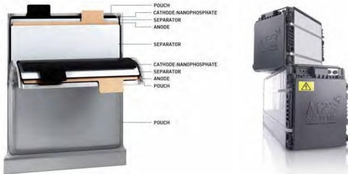
Figure 2-5 | Typical Li-ion prismatic cell design and battery modules (A123, IEC MSB/EES Workshop, 2011)
