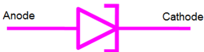
Tunnel diode symbol
