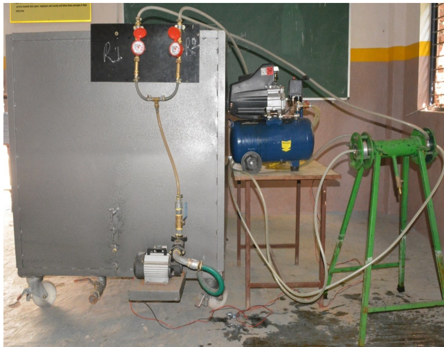
Hydrodynamic Cavitation Treatment Assembly experimental set up
